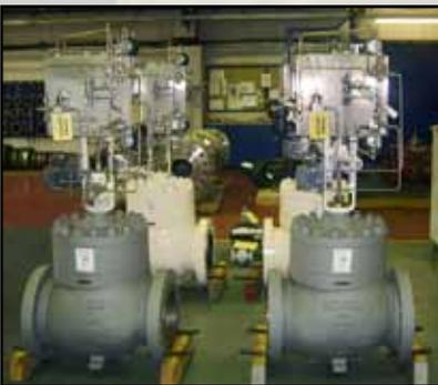
Four compressor recycle valves supplied to BP's Dimlington gas terminal.
